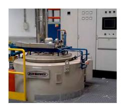
Gas nitriding and ferritic nitrocarburizing require ammonia gas. The ZeroFlow® method was developed by SECO/WARWICK to simplify the nitriding process through the economical use of only raw ammonia (NH<sub>3</sub>). The control of the nitriding atmosphere chemical composition, and therefore the control of nitriding potential (Np), is performed automatically via the ZeroFlow software and hardware controls.
