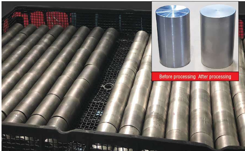
Figure 6. Parts positioned in a basket to illustrate as-quenched surface appearance: (a) atmosphere IQ parts on the left, and (b) Super IQ parts on the right.
