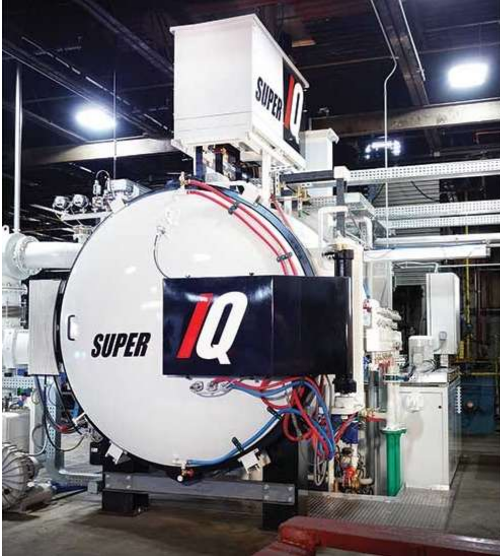
Figure 2. Super IQ furnace – heat chamber with rear maintenance door
