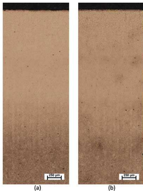
Figure 4. Surface-to-core microstructure: (a) atmosphere IQ, (b) Super IQ (100X, 2% Nital)
