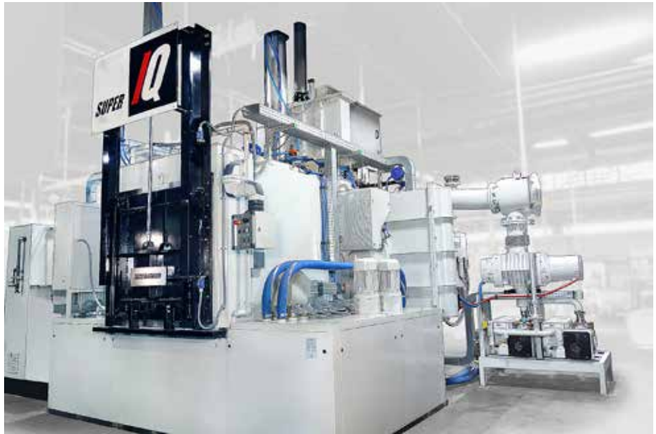
Figure 2: The new atmosphere integral quench furnace (batch in-out style), known as Super IQ™.
