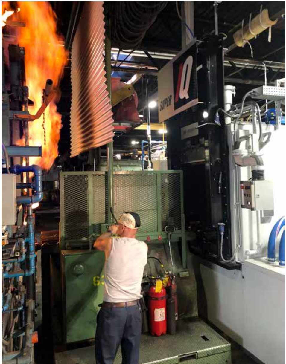
Figure 6: Shared loader with decades-old existing gas carburizing integral quench furnace and modern Super IQ™.
