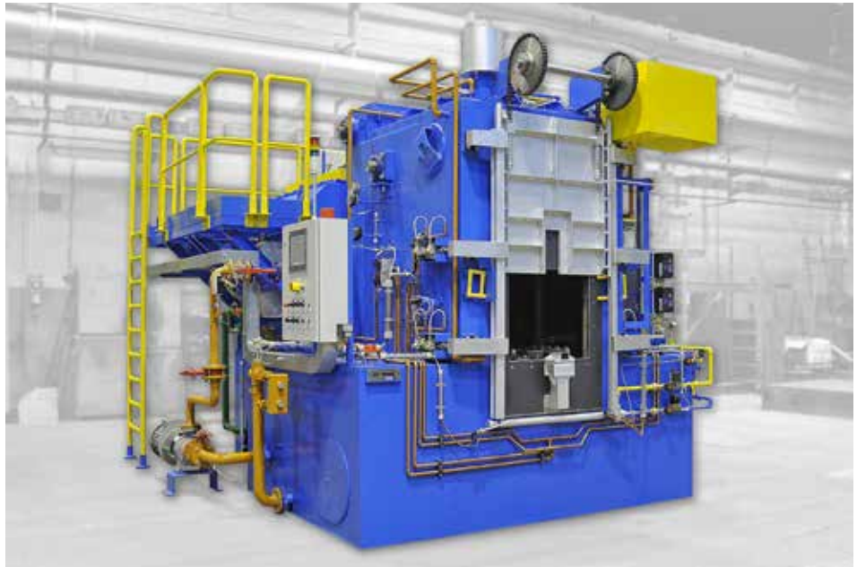
Figure 3: Typical atmosphere integral quench furnace (batch in-out style) with radiant tube fired heating.
