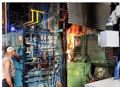
Figure 1. Atmosphere oil quenching
