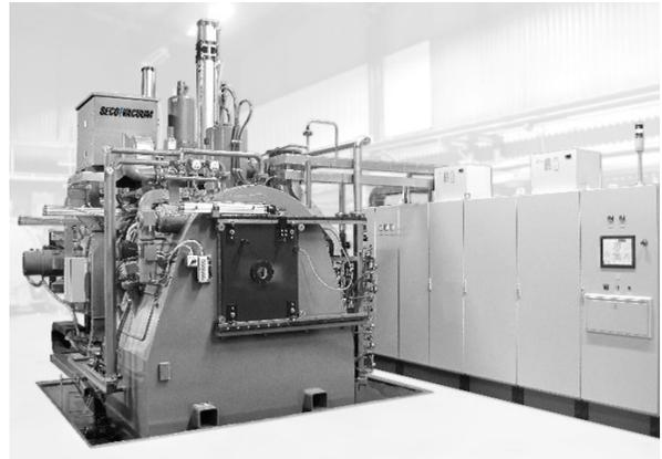
Figure 2. D-Type double chamber for batch work processing with conventional loading over the oil quench
