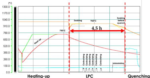
Figure 4. An LPC process that yielded a net 1,322 lb (600 kg) load of gears with an effective case depth of 0.039 in (1 mm). This resulted in a throughput of 294 lb/hr (133 kg/hr). Slight adjustments to this process have rendered production of up to 440 lb/hr. (Source: Maciej Korecki, "Case Study of CMe-T6810-25")
