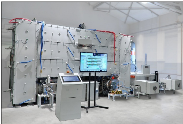
Figure 16 – Single-piece flow vacuum furnace with LPC and with part dedicated HPGQ Chamber [7]
