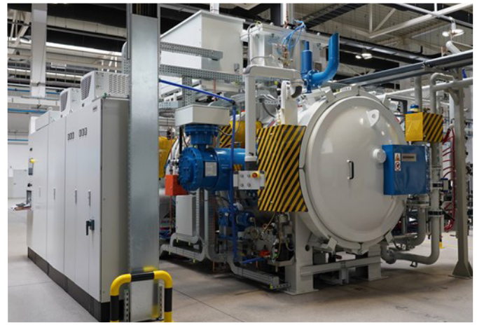
Fig.1. Furnace CMe-T6810-25. On the right – view from the loading side (pre-heating chamber), on the left – view from the unloading side (quenching chamber).
