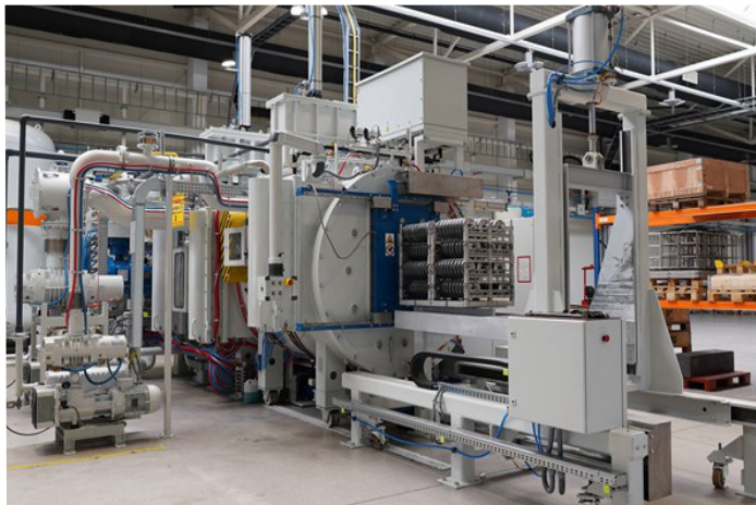
Fig.1. Furnace CMe-T6810-25. On the right – view from the loading side (pre-heating chamber), on the left – view from the unloading side (quenching chamber).
