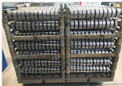
Fig. 5. A photograph of the arrangement of gearwheels in the load.
