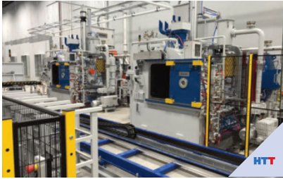
Figure 6: This automated batch line is for low pressure carburizing and vacuum hardening, with oil quench, automated washer, and batch temper furnace. The smart loader makes the cell fully automated.
