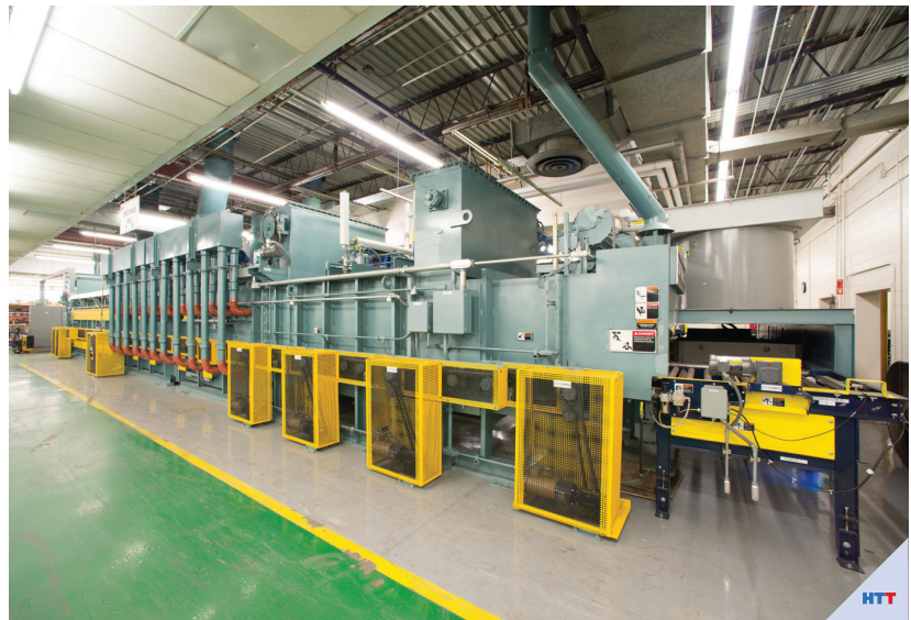
Figure 1: Roller hearth conveyor furnace with heating section, cooling tunnel and after cooling. Note the right angle turn via automatic conveyors to meet space requirements.
