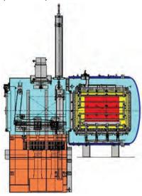
• **D-Type** Double chamber for batch (In & Out) work processing Oil quench or gas cooling/quenching
